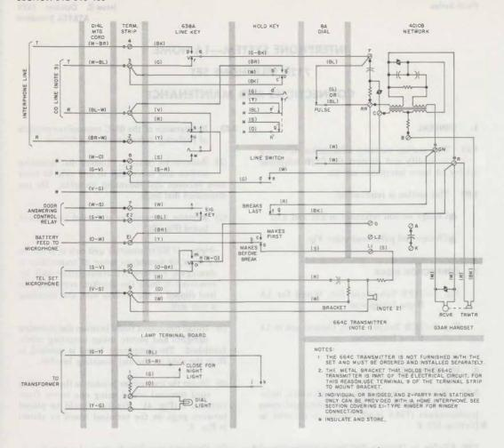
Fig. 1-712B Telephone Set, Wired for 1A Home Interphone
