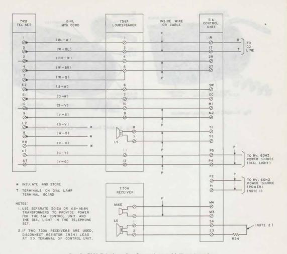
Fig. 2—712B Telephone Set, Connections to 1A Home Interphone
