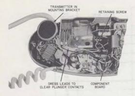
Fig. 3—664C Transmitter, Installed
