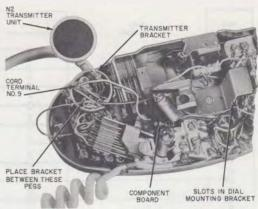
Fig. 4—664C Transmitter, Component Positioning
