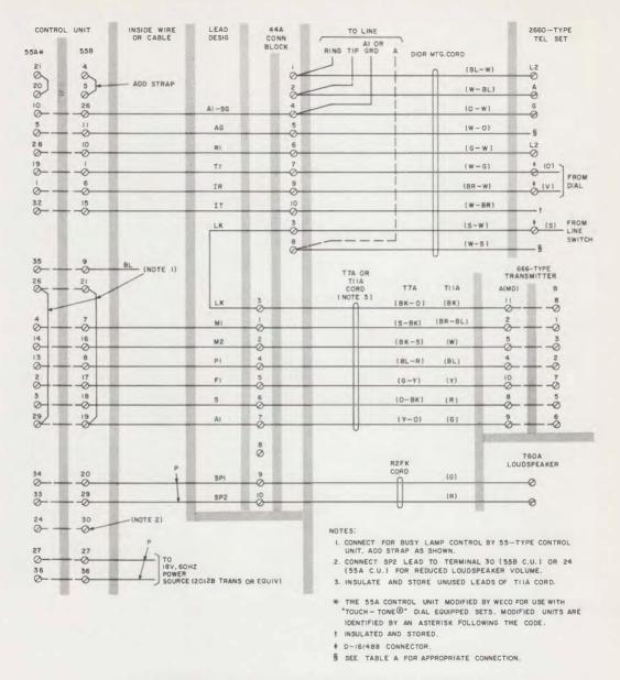
Fig. 2—2660-Type Telephone Set, Connections To 3-Type Speakerphone
