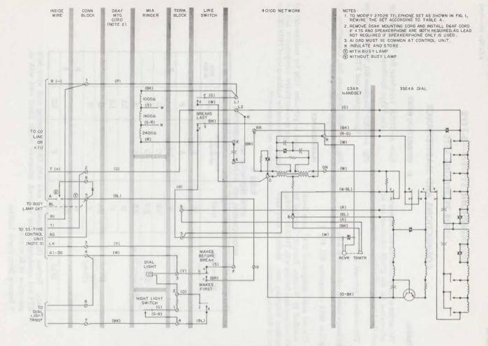
Fig. 1—2702B Telephone Set, Wired For 3-Type Speakerphone and KTS Use
