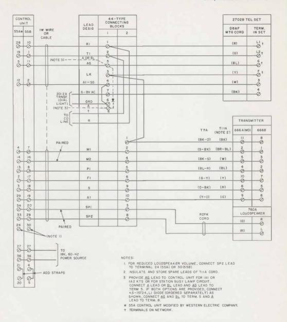
Fig. 2-\$2702B Telephone Set, Connections To 3-Type Speakerphone
