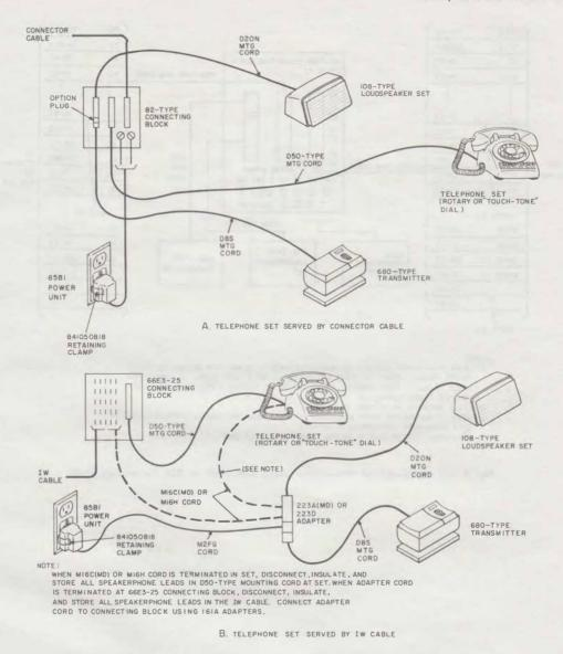
Fig. 1-4A Speakerphone Arrangements, 6-Button Key Telephone Set
