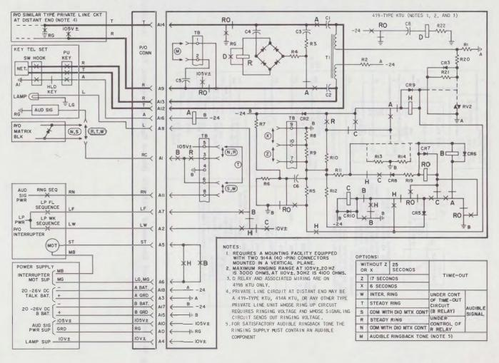
Fig. 14—PCondensed Functional Schematic of 419-Type KTU (Automatic Signaling, Ringdown, Private Line Circuit)
