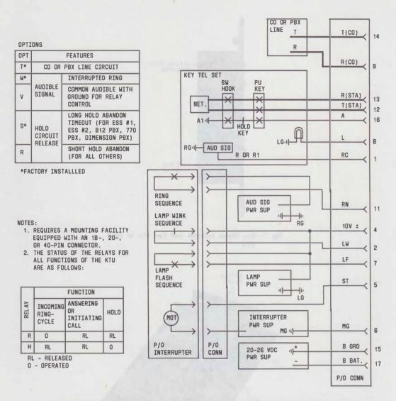
Fig. 9—Condensed Functional Schematic of 400H KTU (CO or PBX Line Circuit) (Sheet 1 of 2)
