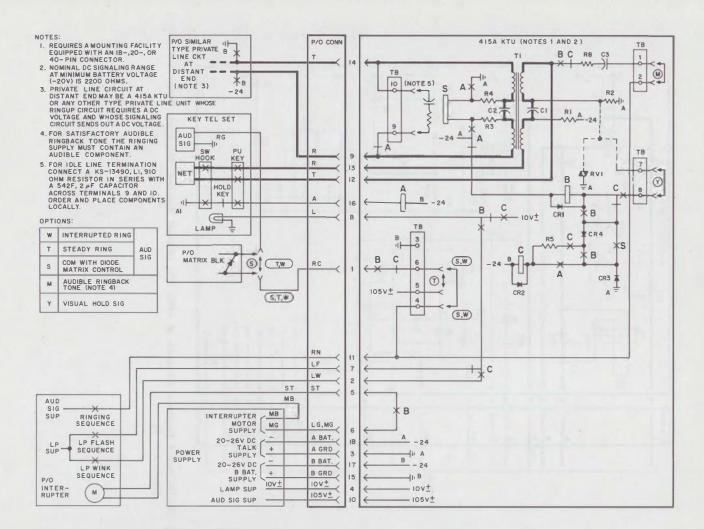
Fig. 11—Condensed Functional Schematic of 41SA KTU (Automatic, DC Signaling, Private Line Circuit)
