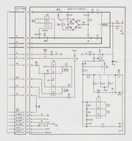
Fig. 15—Condensed Functional Schematic of 461A KTU (Manual Signaling, Ringdown, Private Line Circuit) (Sheet 2 of 2)
