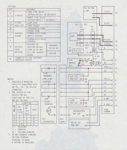
Fig. 6—Condensed Functional Schematic of 400G KTU (CO or PBX Line Circuit) (Sheet 1 of 2)
