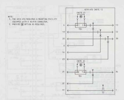
Fig. 9—♦Condensed Functional Schematic of 421A KTU (General Purpose Relay)♦
