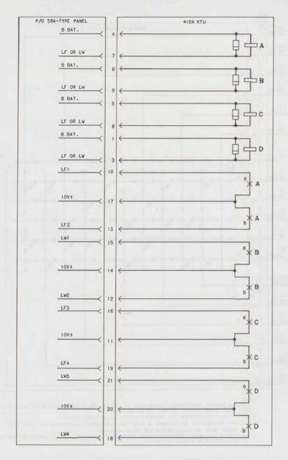
Fig. 5— Condensed Functional Schematic of 412A KTU (Auxiliary Relay Circuit)
