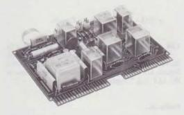
Fig. 2—Typical 8-Inch Key Telephone Unit
