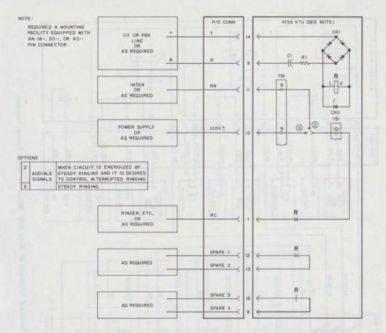
Fig. 6—Condensed Functional Schematic of 413A KTU (Auxiliary Ringup Circuit)
