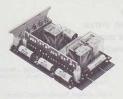
Fig. 1—Typical 4-Inch Key Telephone Unit
