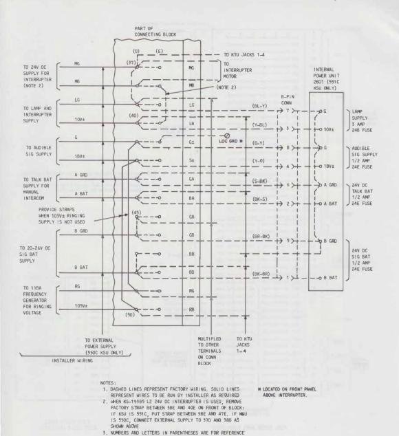
Fig. 5—Power Supply Connections for 550/551C KSU
