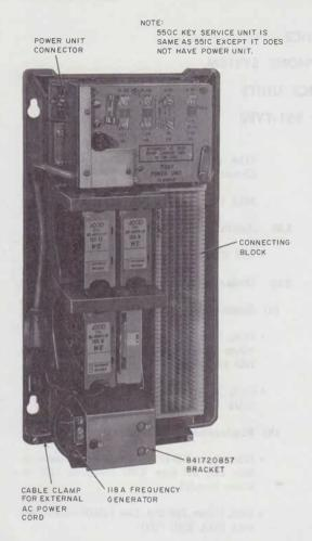
Fig. 1-551C KSU With Frequency Generator
