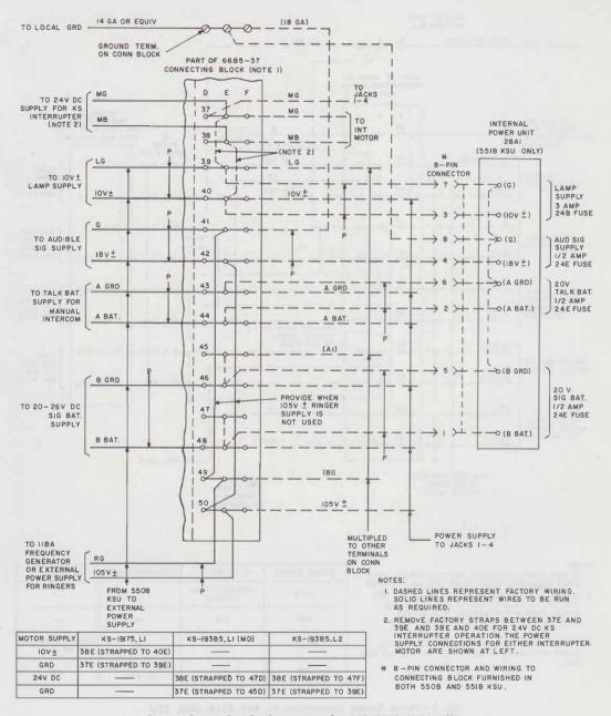
Fig. 6—Power Supply Connections for 550/551B (MD) KSU
