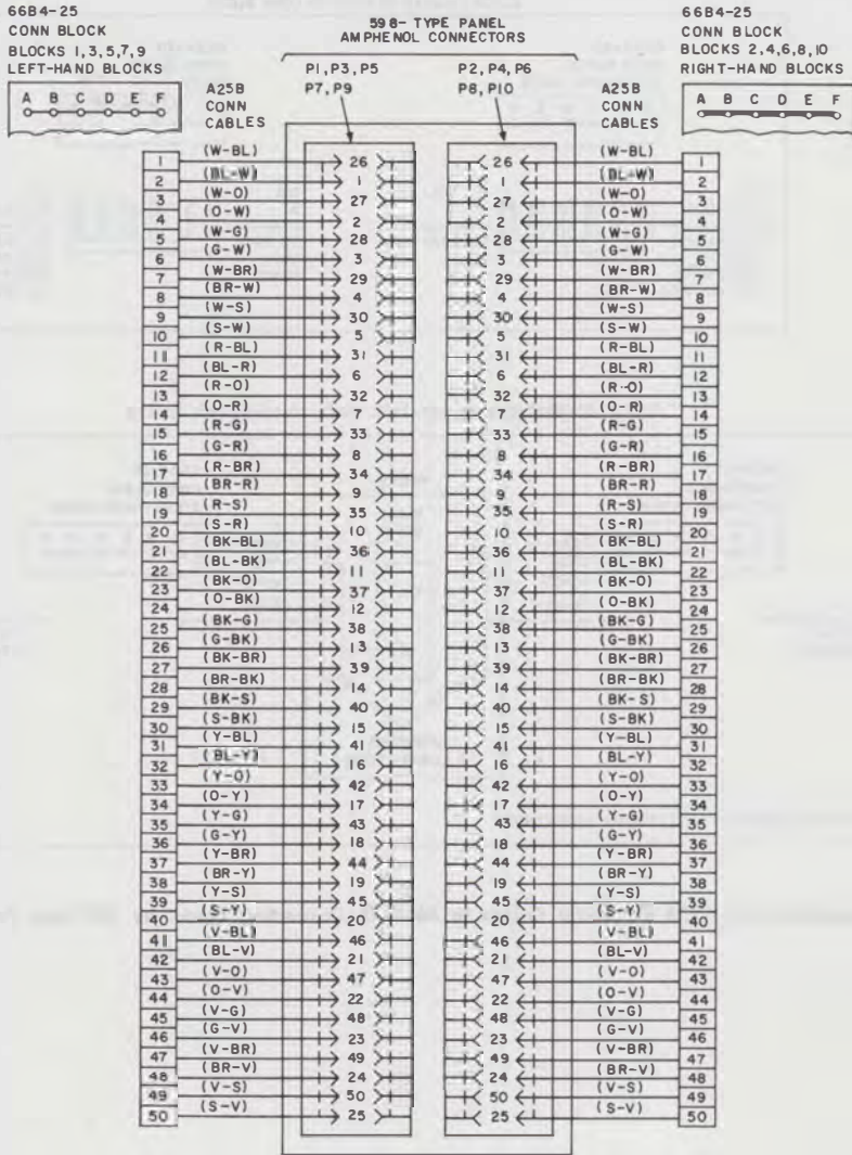
Fig. 6—Connections for A25B Connector Cables to 66B4-25 Connecting Blocks for 598-Type Panel (Sheet 1)
