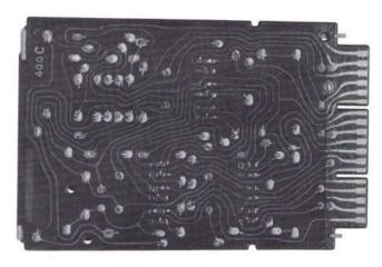
Fig. 2 — 400C Key Telephone Unit
