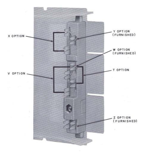
Fig. 5 — Option Block, 400A, B, and C KTUs
