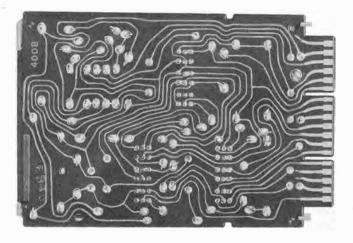
Fig. 1 — 400B Key Telephone Unit
