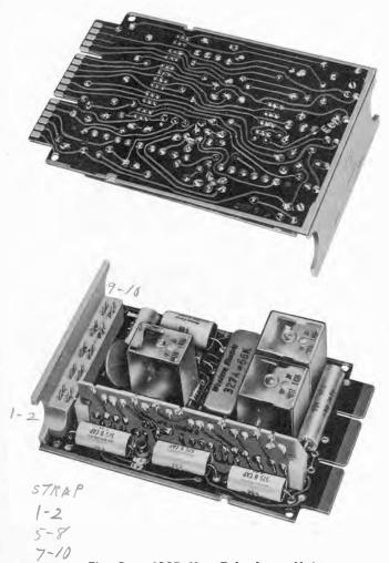
Fig. 3 — 400D Key Telephone Unit
