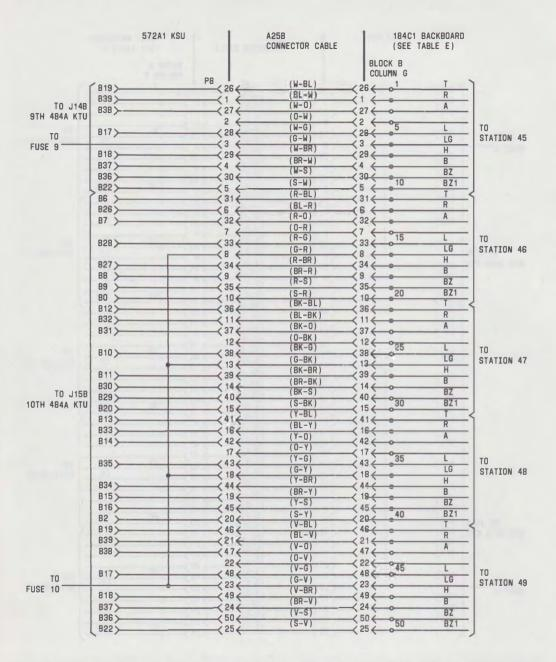
Fig. 33—Connections Between Plugs 5 to 8 of 572A1 Key Service Unit and 184C1 Backboard (Sheet 4 of 4)
