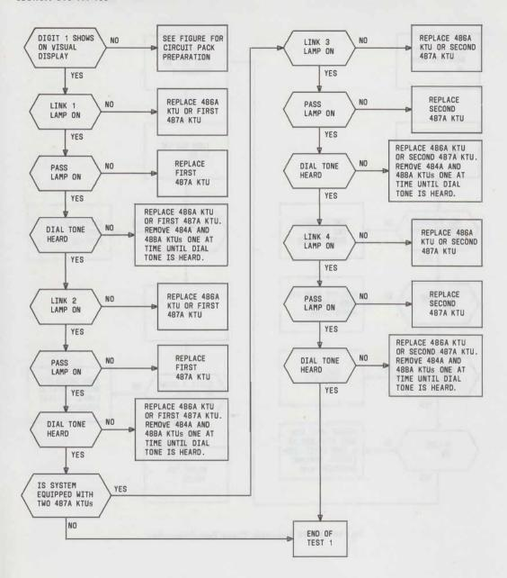
Fig. 20—Test 1 Sequence—Link Operation and Dial Tone
