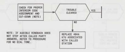
Fig. 15—Cannot Call Specific Station—Audible Ringback Heard
