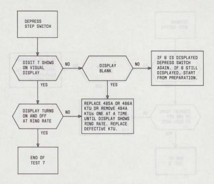
Fig. 26—Test 7 Sequence—Ring Rate
