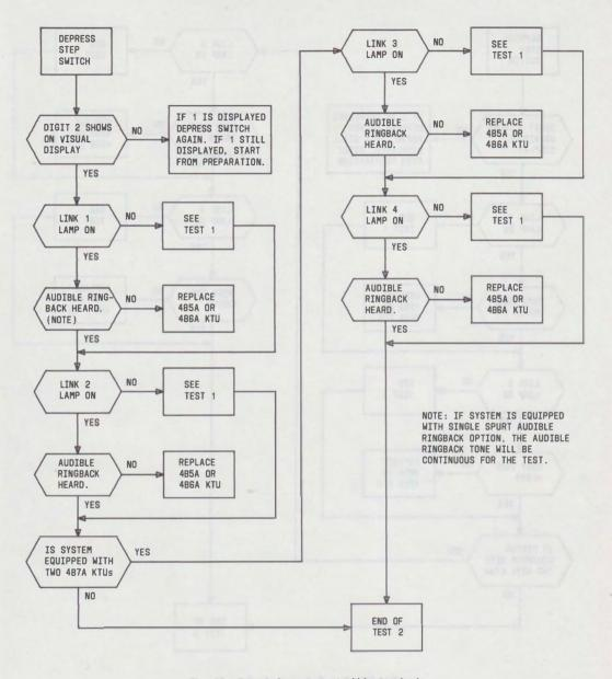
Fig. 21—Test 2 Sequence—Audible Ringback
