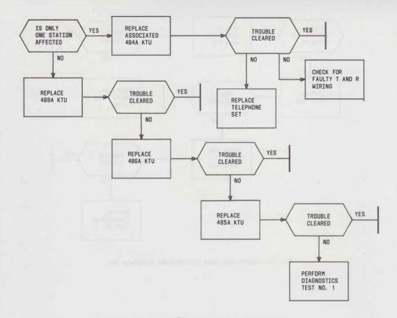
Fig. 12—Cannot Dial From Rotary Dial Telephone Set
