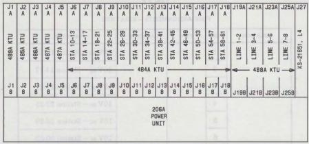
484A KTU-STATION CIRCUIT 485A KTU-CONTROLLER CIRCUIT 486A KTU-SERVICE CIRCUIT 487A KTU-BATTERY FEED CIRCUIT
