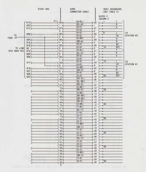
Fig. 34—Connections Between Plugs 9 to 11 of 572A1 Key Service Unit and 184C1 Backboard (Sheet 3 of 3)
