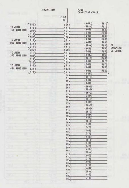
Fig. 31—Terminations of Incoming CO/PBX Lines in 572A1 KSU
