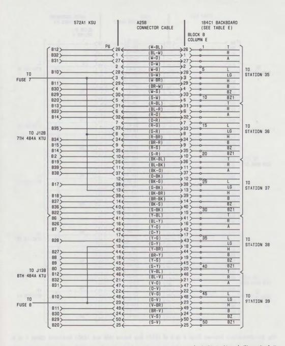
Fig. 33—Connections Between Plugs 5 to 8 of 572A1 Key Service Unit and 184C1 Backboard (Sheet 2 of 4)
