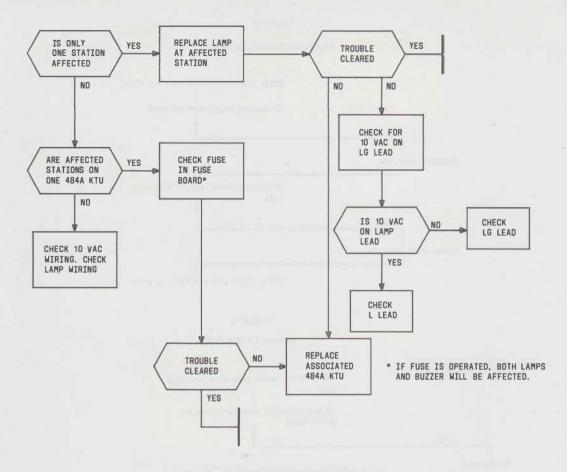
Fig. 9—Intercom Lamp Does Not Light
