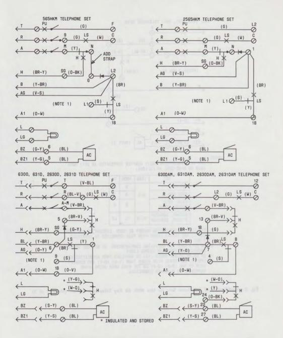
Fig. 3-Modification of Telephone Sets for Use With 6B Key Telephone System (Sheet 1 of 2)
