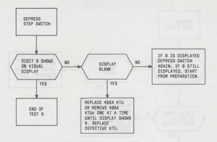
Fig. 28—Test 9 Sequence—Slow CO Disconnect
