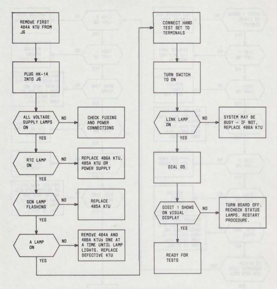
Fig. 19—HK-14 Diagnostic Circuit Pack Preparation
