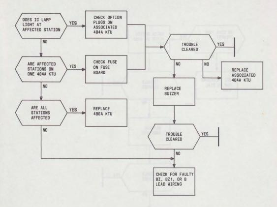
Fig. 13-Intercom Buzzer Does Not Operate
