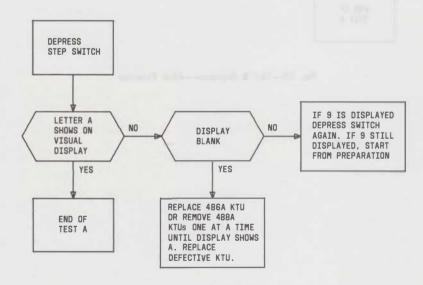
Fig. 29—Test A Sequence—Fast CO Disconnect
