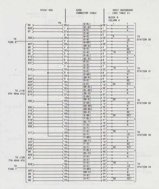
Fig. 33—Connections Between Plugs 5 to 8 of 572A1 Key Service Unit and 184C1 Backboard (Sheet 1 of 4)
