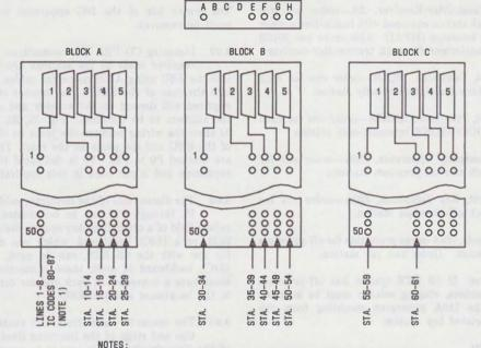
1. CONNECTOR 1 ON BLOCK A IS CONNECTED TO P12 ON REAR OR KSU.
