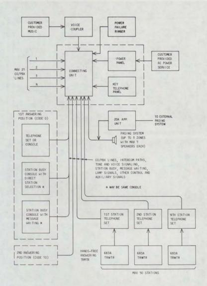
Fig. 1—Block Diagram of 21A Communication System
