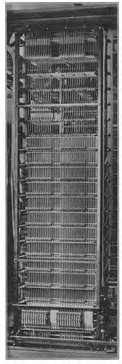
Figure 5. Line finder frame showing multiple banks and selecting mechanisms.
