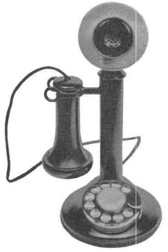
Figure 1. Telephone equipped with dial.
