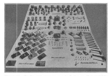
Figure 23. Tools and gauges required for making multiple brushes. One of these brushes appears in the foreground and is also shown in Fig. 24.
