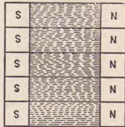
End view of magnets of a 5-bar generator with bars placed wrong.
