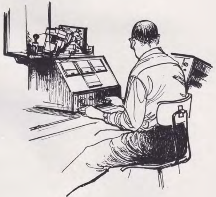
Picturephone display units being assembled and tested at Western Electric's Indianapolis plant. Among the many operations: mounting the picture tube and frame assembly on the ring stand (top left), checking circuit boards visually (top right), placing them in the display unit (bottom left), and finally, testing for picture alignment.
