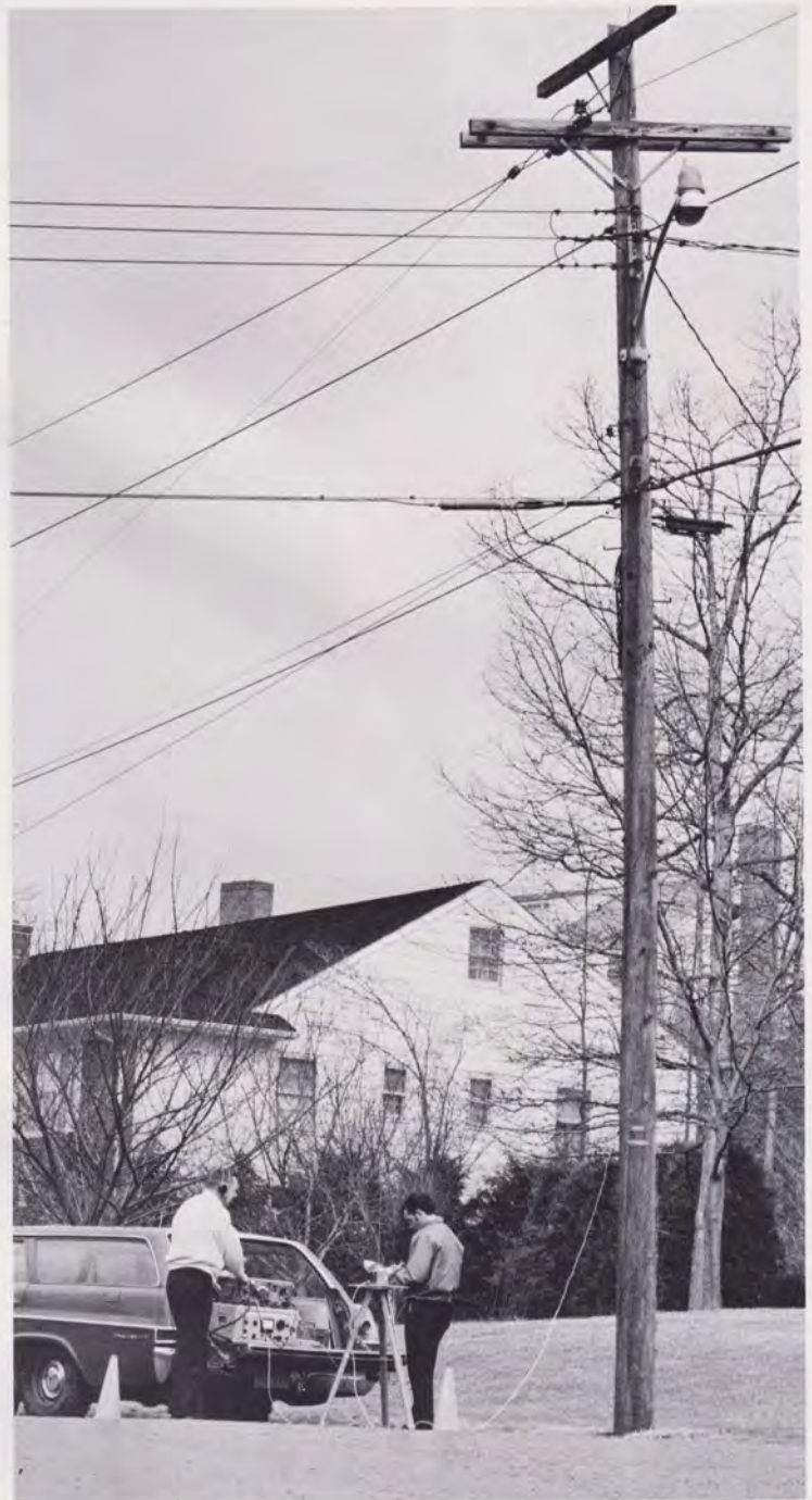
M. F. Veverka and E. W. Banz, Jr., both of Bell Laboratories, measure electric field strength and the associated interference on telephone lines to help determine the need to prevent radio frequency interference with the 1-MHz video signal.
