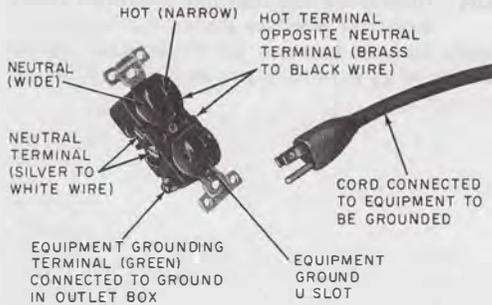
Fig. 8—Wiring of 125V Standard Plug and Receptacle
