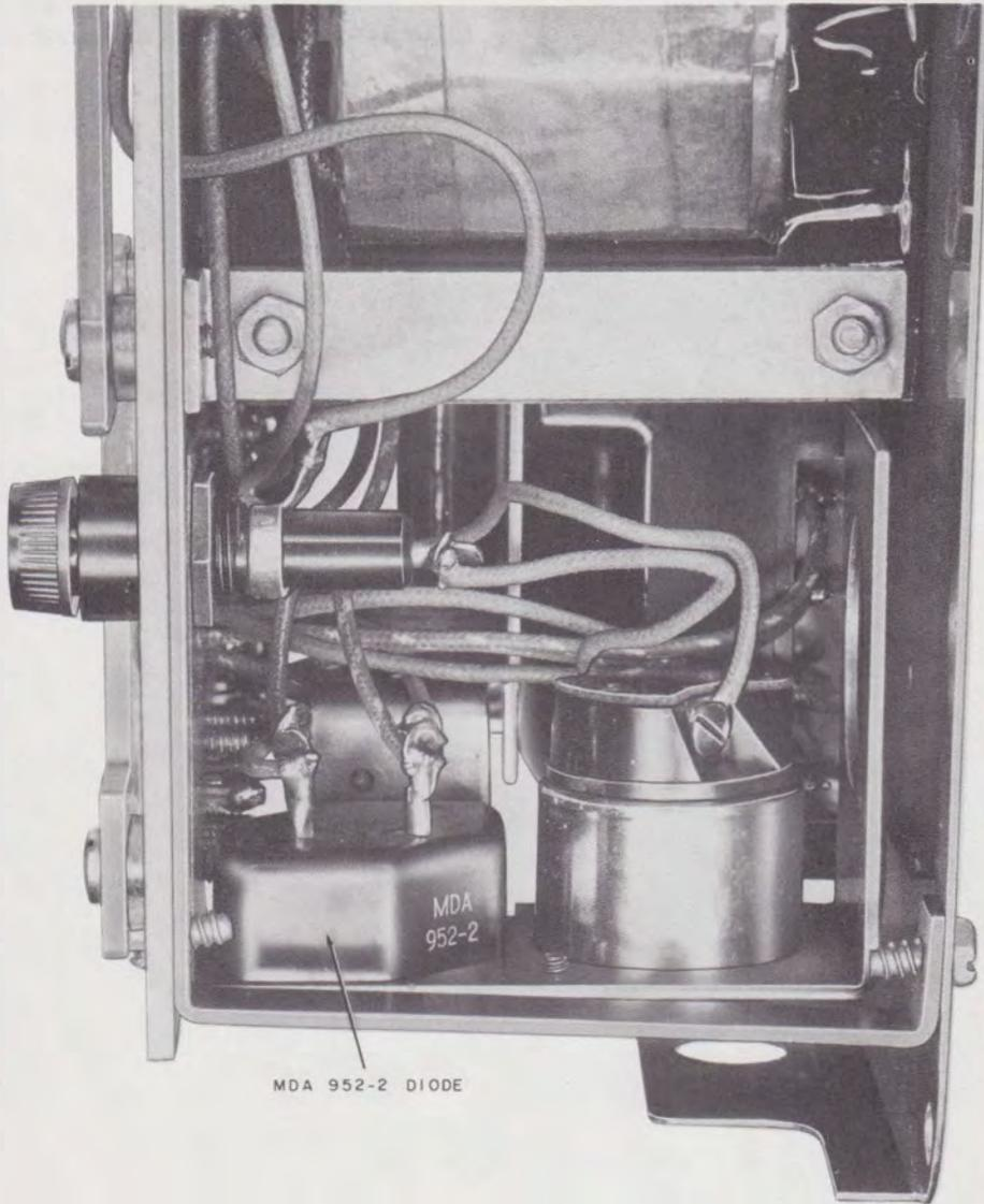
Fig. 6—Diode Location on 20B1 Power Unit
