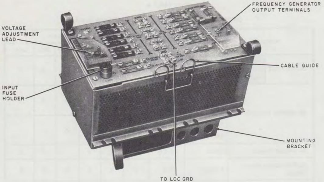
Fig. 3—30C1 Power Unit (Rack Mounted) Cover Installed
