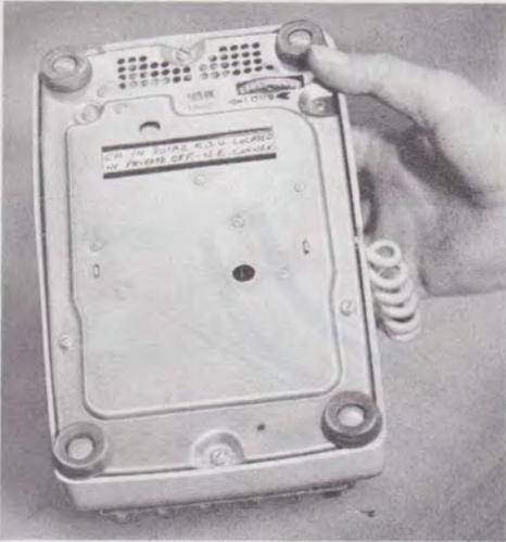
Fig. 3—Marking Equipment Location Using Form E-5826
