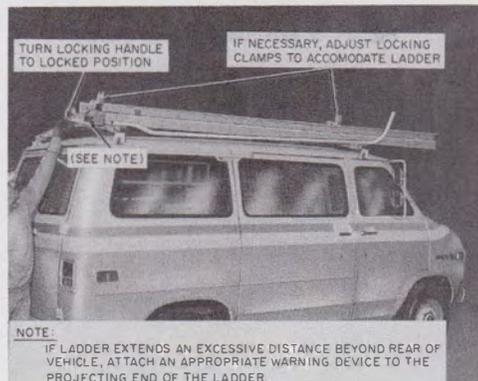
Fig. 4—Mounting Ladder on Roof-Type Ladder Bracket
