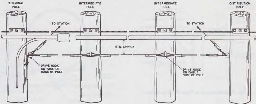
Fig. 4—Drop Wire Run Along Lead Carrying Cable
