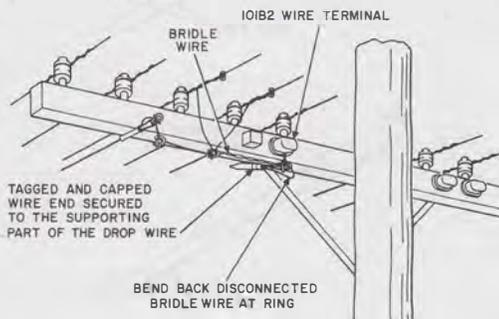
Fig. 8—Wire Terminal Mounted on Crossarm
