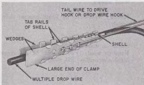
**Fig. 2—D Drop Wire Clamp Assembled on Wire**
