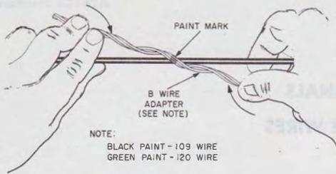
Fig. 9 - Installation of B Wire Adapter
