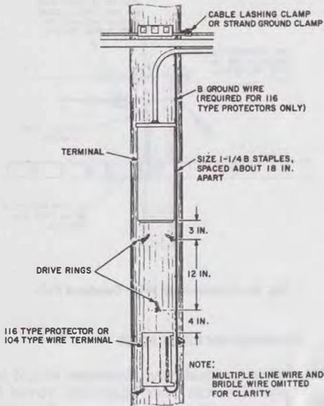
Fig. 10—Pole With Pole-Mounted Cable Terminal (multiple line wire and bridle wire omitted for clarity)
