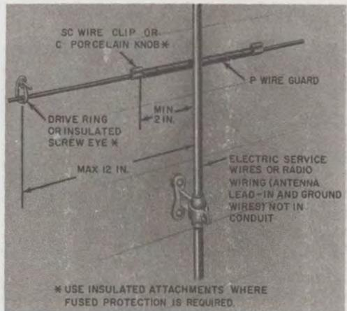
Fig. 9—Wires Crossing Power, Radio, or Television Wires on Wood, Stucco, or Metal Siding
