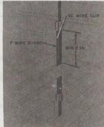
Fig. 5—Protecting Wire Run Through Stationary Metal Grating
