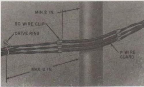
Fig. 6—Wires Crossing Downspout on Masonry or Brick Surface
