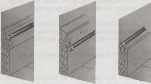
**Fig. 6—Wiring to Baseboards**
