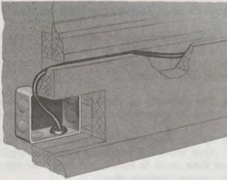
**Fig. 5—Wiring From Conduit to Baseboards**
