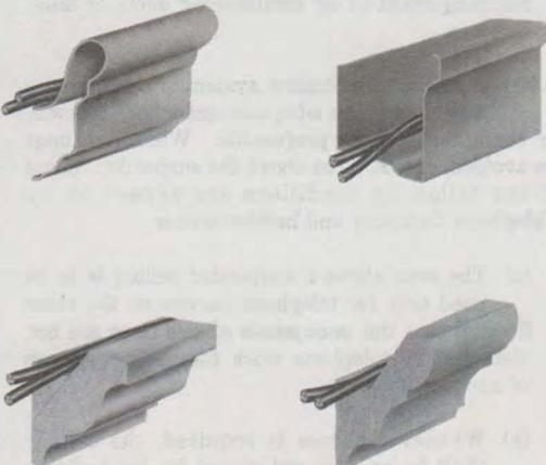
**Fig. 7—Wiring in Picture Moldings**
