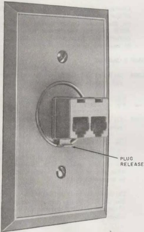
Fig. 13.1—267A Adapter (Plugged Into 625B Connecting Block)
