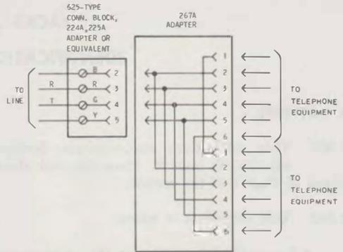
Fig. 13.2—Schematic Diagram, 267A Adapter
