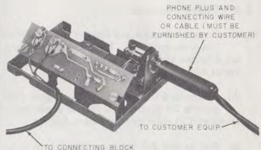
Fig. 2—30-Type Voice Coupler, Cover Removed
