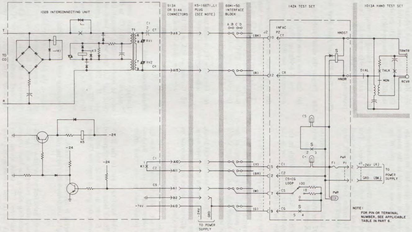
Fig. 14—Testing 102B Interconnecting Unit With 142A Test Set
