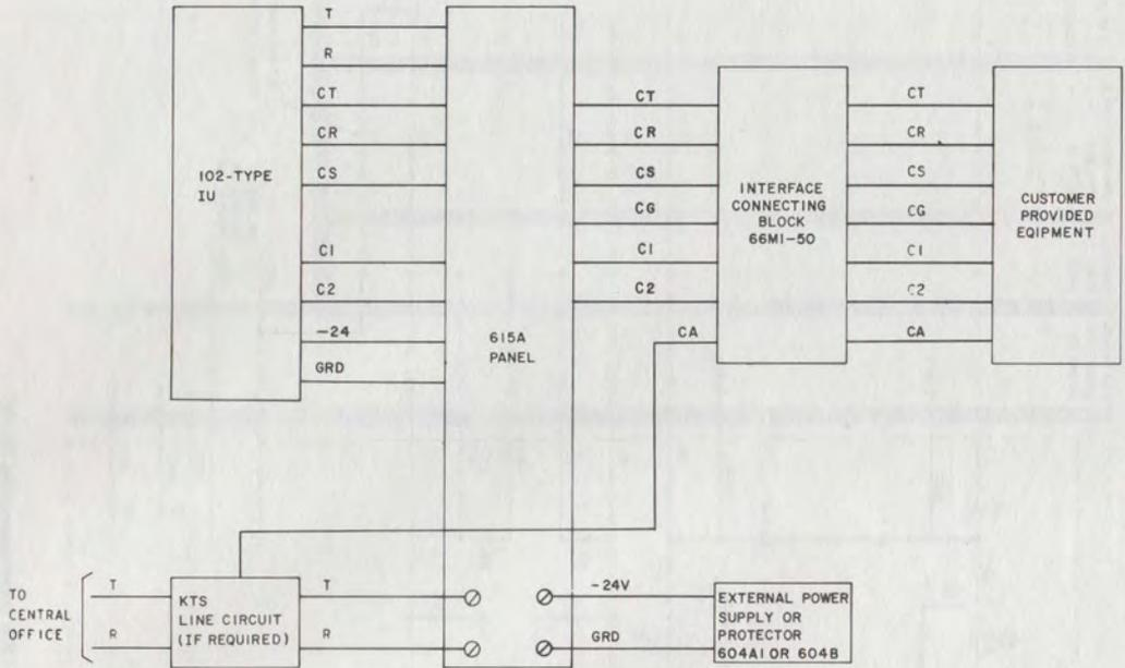
Fig. 11—Block Diagram—102-Type Interconnecting Unit with 615A Panel
