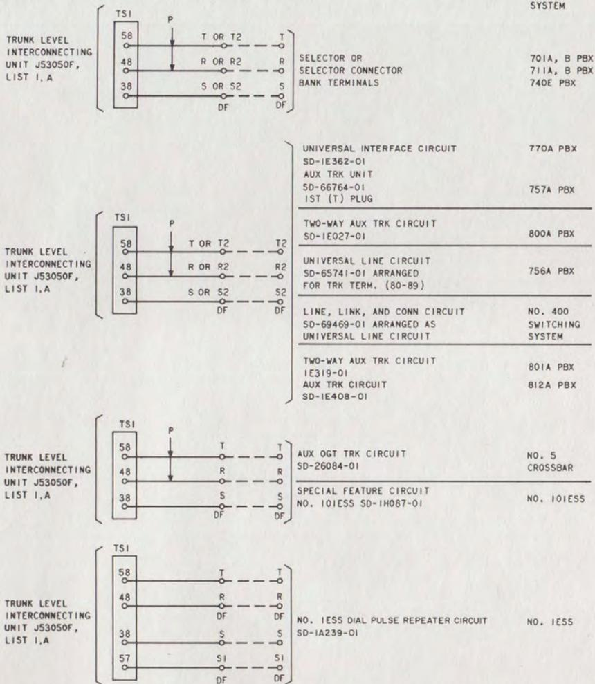
Fig. 5—Typical Connections for System Terminating Circuits with Trunk Level Interconnecting Unit J53050F, List 1
