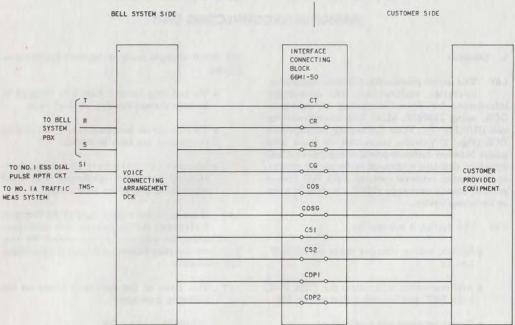
Fig. 2—Block Diagram—Voice Connecting Arrangement DCK
