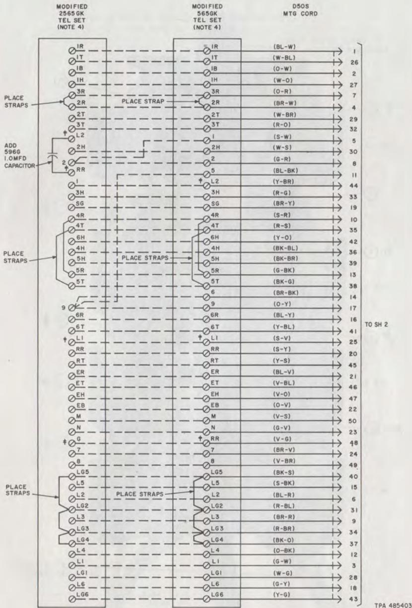
Fig. 10—Connections Using KS-16765, List 1 Announcement Set, KS-19522 Recorder Coupler and 565GK or 2565GK Telephone Set With Customer-Provided Message Recorder (Sheet 1)
