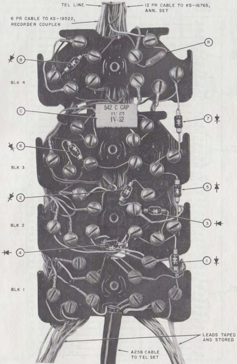
Fig. 9—44A Connecting Blocks With Components Mounted
