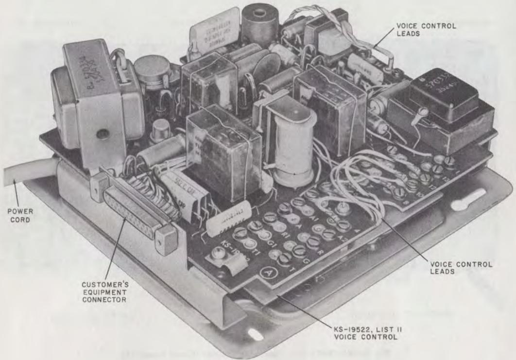
Fig. 3—KS-19522, List 2 Recorder Coupler (Cover Removed)
