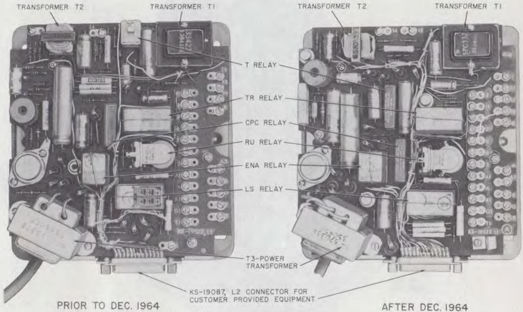
Fig. 2—KS-19522, List 1 Recorder Coupler (Cover Removed)
