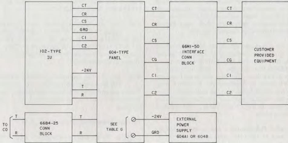
Fig. 7—Block Diagram—102-Type Interconnecting Unit With 604-Type Panel
