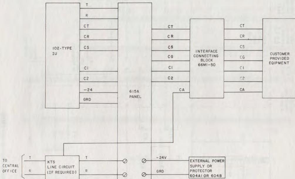
Fig. 8—Block Diagram—102-Type Interconnecting Unit With 615A-Type Panel
