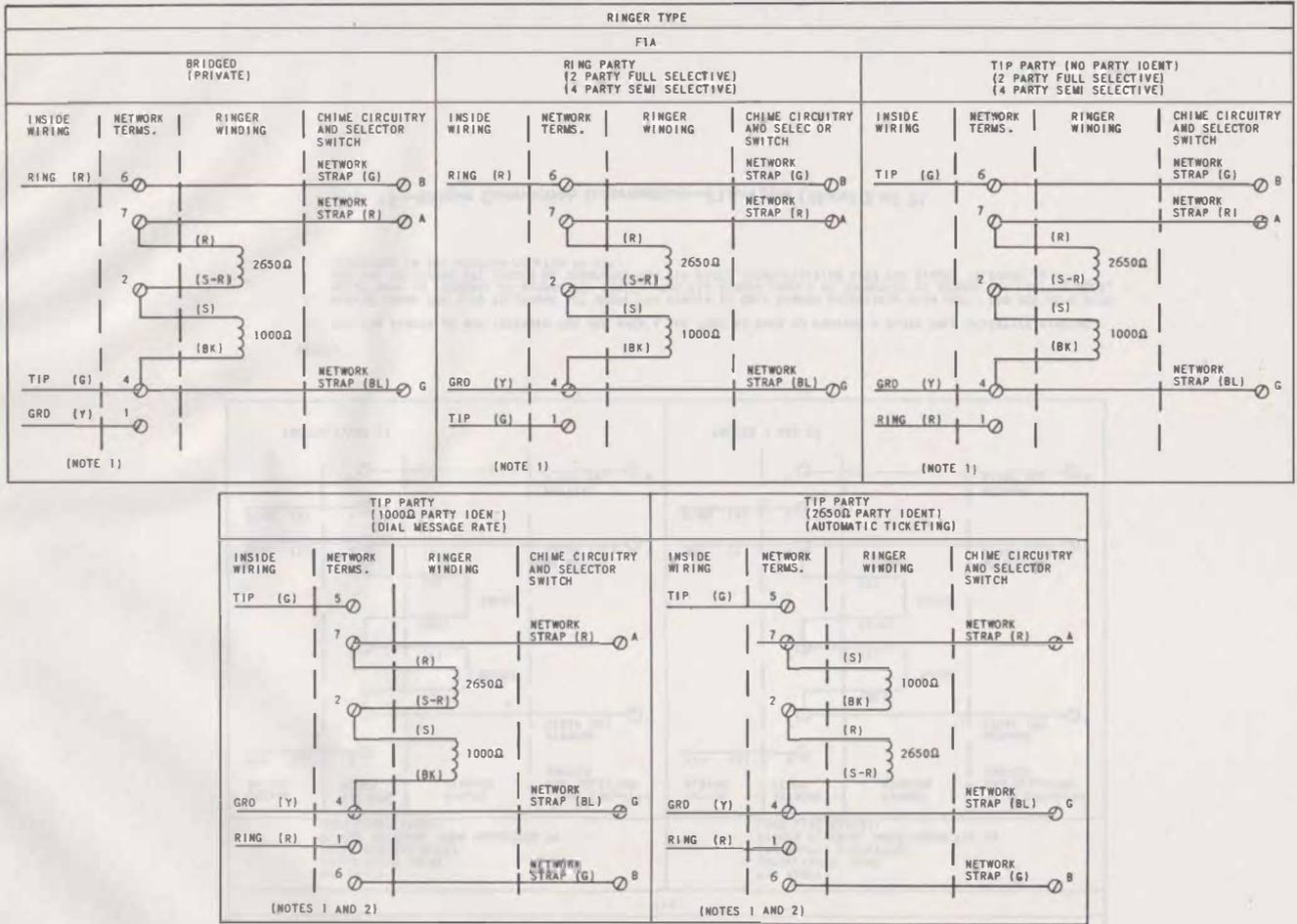
Fig. 11—Ringer Connection Information—FIA-Type (Sheet 1 of 2)
