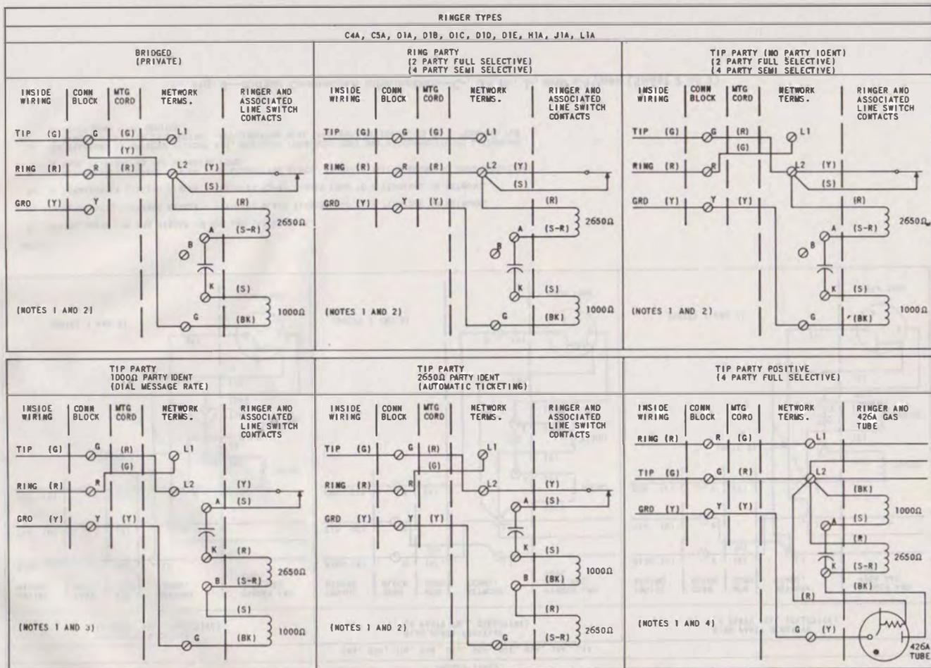
Fig. 8—Ringer Connection Information—C-, D-, H-, J-, and L-Types (Sheet 1 of 2)
