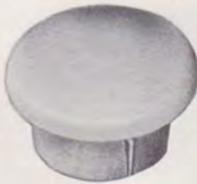
**Fig. 11—93C**—White finished wooden blank, 13/16-inch long by 1-7/64 inches in diameter. For plugging 1-1/8 inch hole in ceiling of telephone booth.
