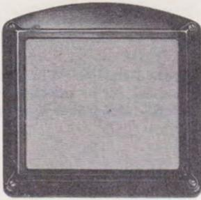
♦**Fig. 8—50K**—Metal mounting plate, 4-11/16 inches high by 4-3/4 inches wide. Equipped with a card frame, card holder assembly, Allen head mounting screws, and plastic window protector for the instruction card. Early production models will be provided with slot head mounting screws, and without the plastic window. The chrome plated 50K apparatus blank replaces the 50L apparatus blank. For all type coin collectors.♦
