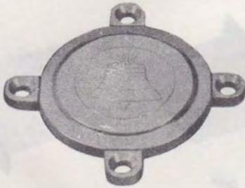
**Fig. 15—108A**—Colored plastic plate; available in light olive gray (-49), brown (-54), and ivory (-50). For covering unused opening in 16A faceplate.
