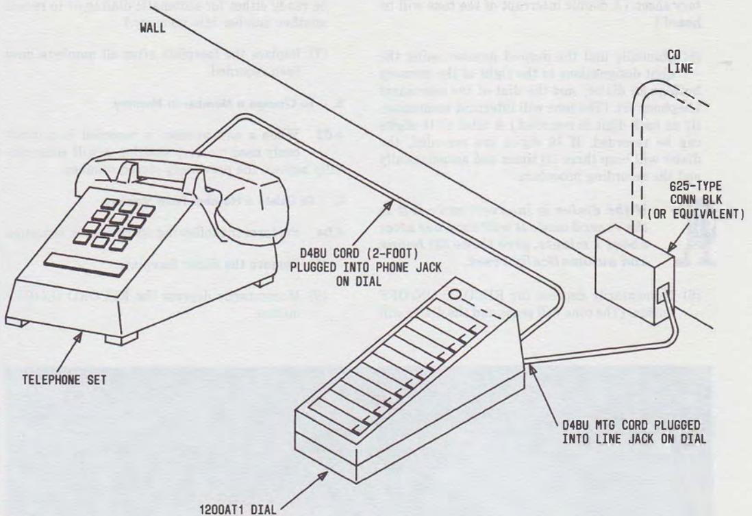
Fig. 5—Recommended Installation Using 1200AT1 Dial
