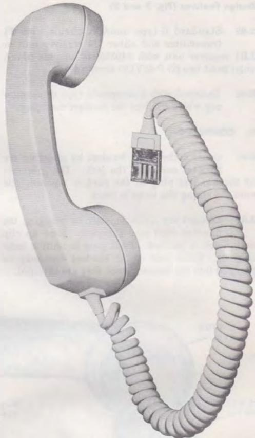
Fig. 1—G12A Handset with Handset Cord Connected
