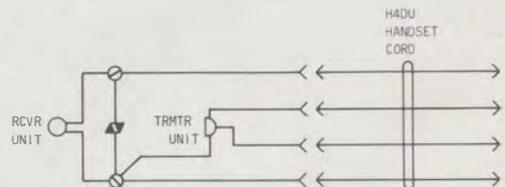
Fig. 2—M1A Handset, Internal Connection
