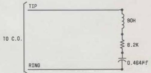
Fig. 2—1A Termination Unit, Connections
