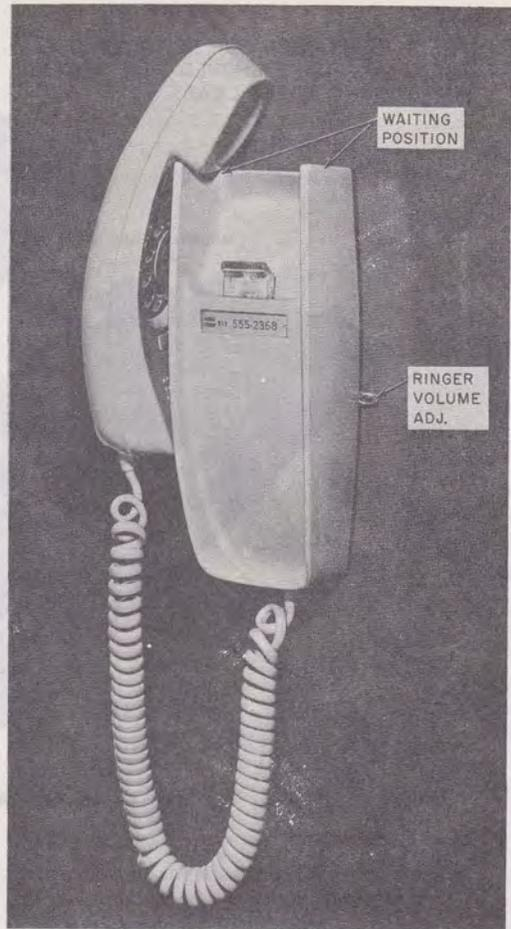
Fig. 7—220A Hand Telephone Set in Waiting Position on AC1 Telephone Base
