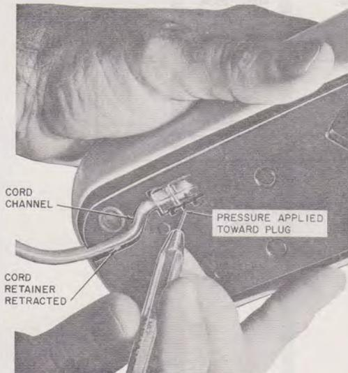
**Fig. 16—Removing Mounting Cord From AD1 Telephone Base**
