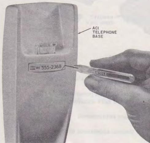
Fig. 6—Removing Number Plate Retainer
