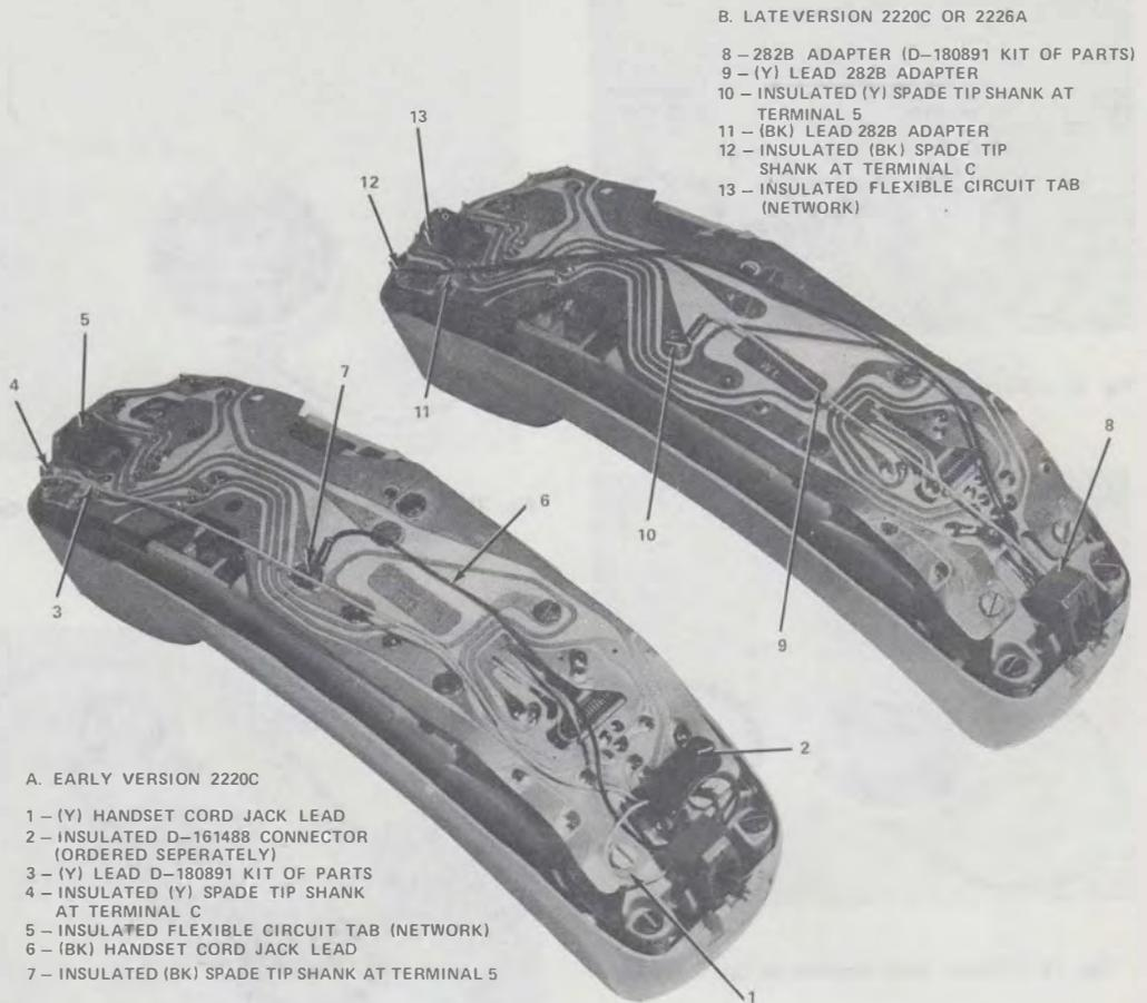
Fig. 10—2220C or 2226A Hand Telephone Set Modified for RFI
