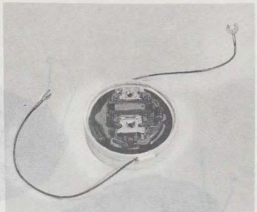
Fig. 13—Receiver Unit and Gasket Installed in Coil Assembly
