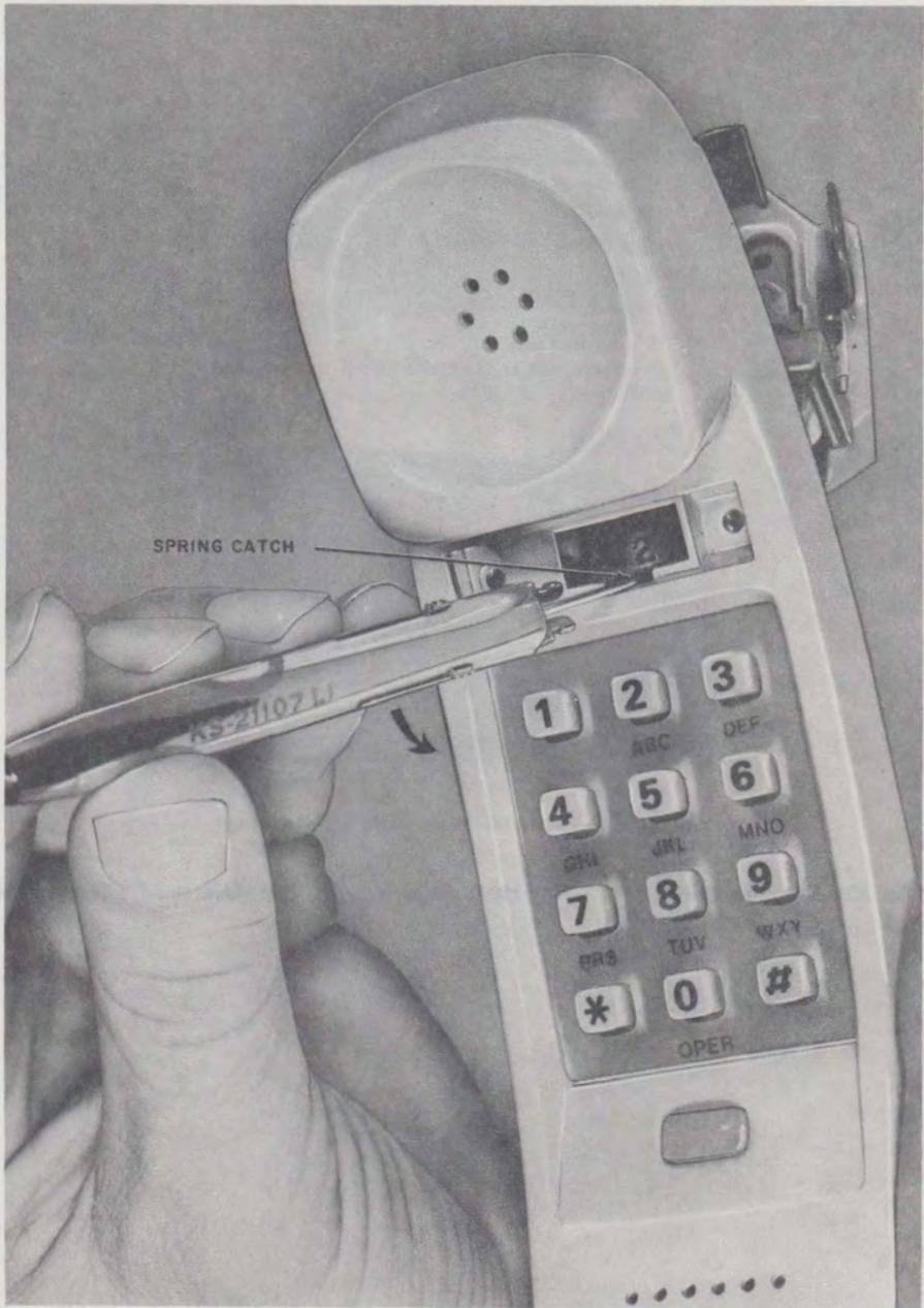
Fig. 21—Releasing Spring Catch on 315-Type Amplifier
