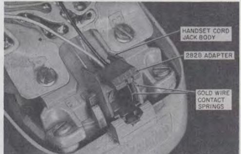
A. INSTALLING 282B ADAPTER ON EXISTING HANDSET CORD JACK
