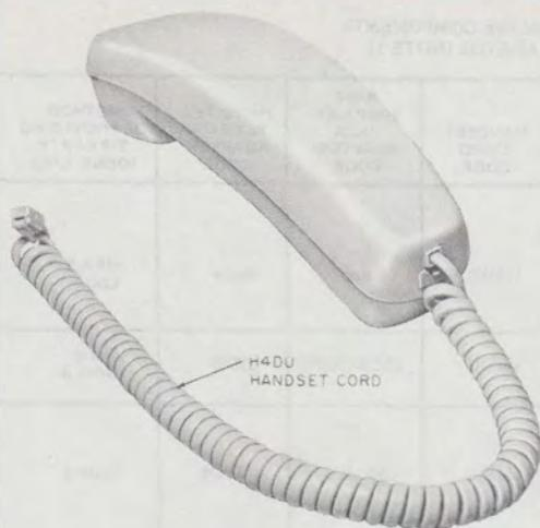
**Fig. 4—H4DU Handset Cord Installed in Hand Telephone Set**
