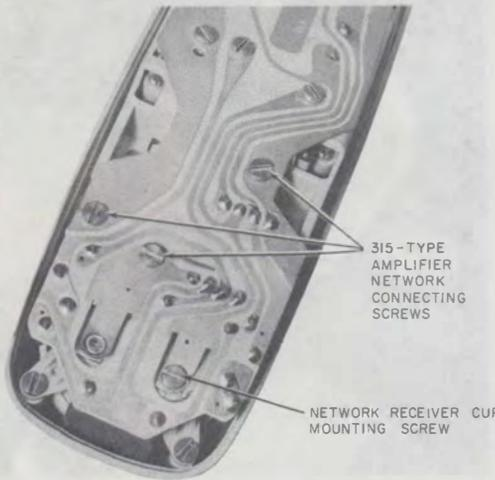
Fig. 19—Location of Mounting Screws Used to Connect Amplifier in Hand Telephone Set
