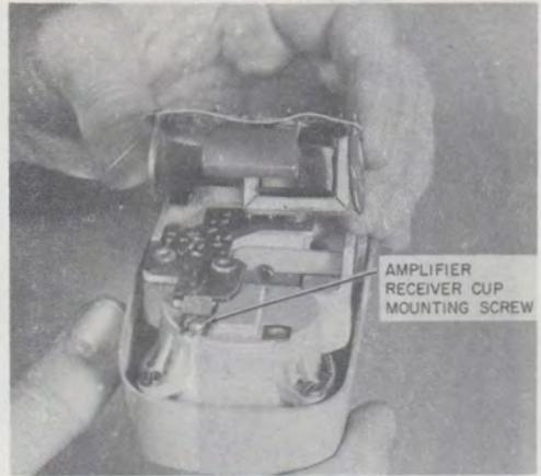
Fig. 20—Fastening Amplifier to Receiver Unit Cup of Hand Telephone Set
