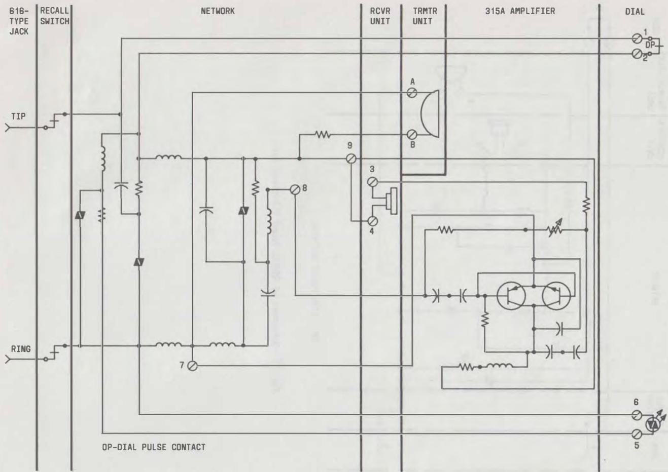
Fig. 26—Schematic of 226A Hand Telephone Set
