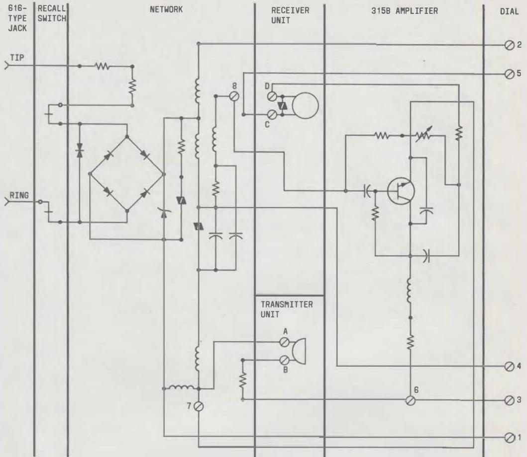
Fig. 29—Schematic of 2226A Hand Telephone Set
