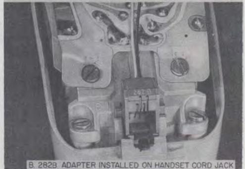
Fig. 9—D-180825 Kit of Parts Installed in 220C, 226A, 2220C, or 2226A Hand Telephone Set
