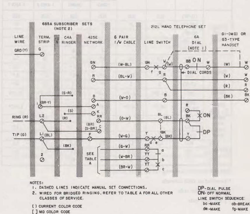
◆ Fig. 1—212L Hand Telephone Set Connections Used with 685A Subscriber Set ◆
