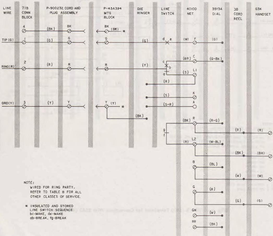
◆ Fig. 1—2750A and B Telephone Set, Connections (Current Model) ◆
