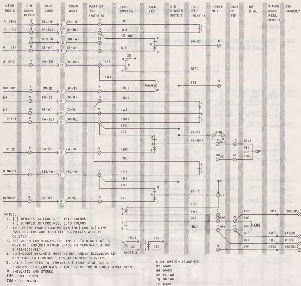
Fig. 2—751C and D Telephone Set Connections
