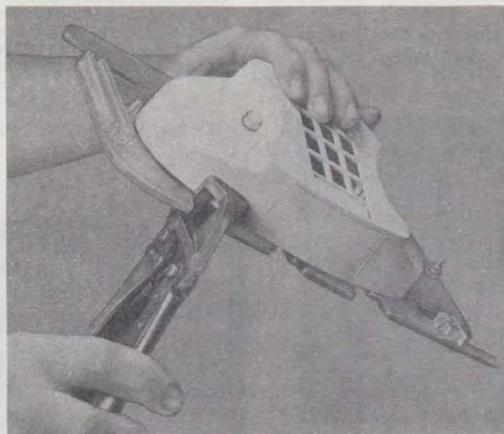
Fig. 53—Notching 2702B1 Housing and Using Check Gauge
