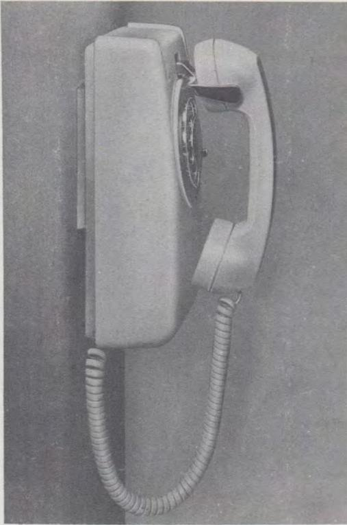
Fig. 35—5548BMP Telephone Set on 630A-Type Connecting Block
