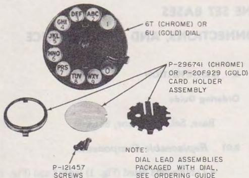
**Fig. 2—6T or 6U Dial and Associated Parts**
