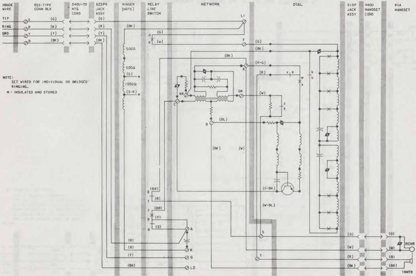
Fig. 8—2900A (MD) Telephone Set, Connections for Nonkey
