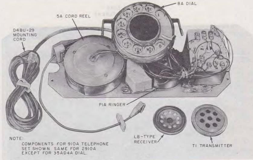
**Fig. 5—Telephone Company-Owned Components**
