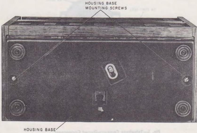
Fig. 6—Removing Metal Housing Base (910A or 2910A Telephone Set)
