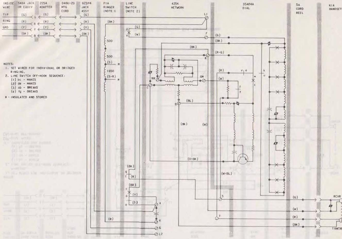
Fig. 10—2910A Telephone Set, Connections
