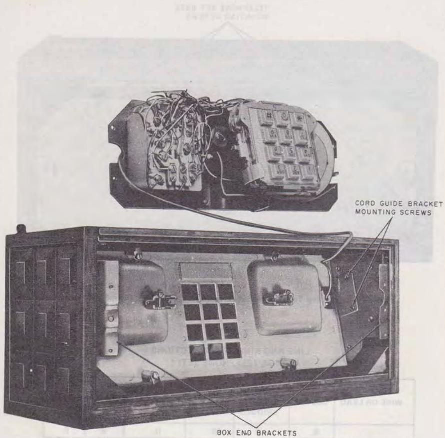
**Fig. 8—Removing Cord Reel Plug from 910A or 2910A Telephone Set**
