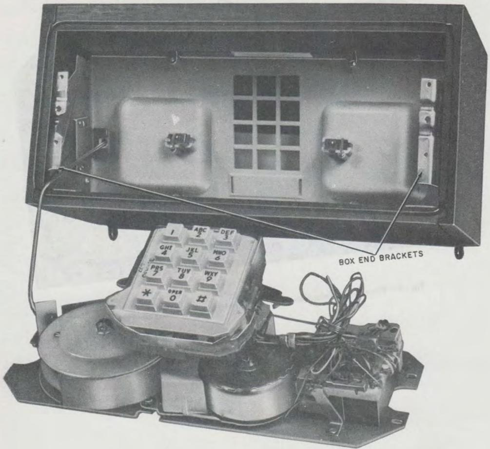
Fig. 6—2910A Telephone Set with Telephone Set Base Removed
