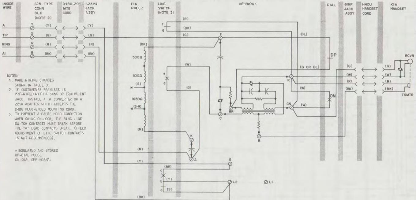
Fig. 10—930A-(MD) or 930B-Type Telephone Set Wired for 1A1 or 1A2 KTS
