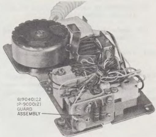
**Fig. 3—819040122 (P-90D012) Guard Assembly (Polarity Guard) Installed on Telephone Set Base**
