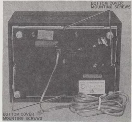
Fig. 4—881C- or 2881C-Type Telephone Set, Bottom View
