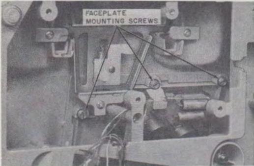
Fig. 8—Removing Faceplate from Set Equipped With TOUCH-TONE Dial
