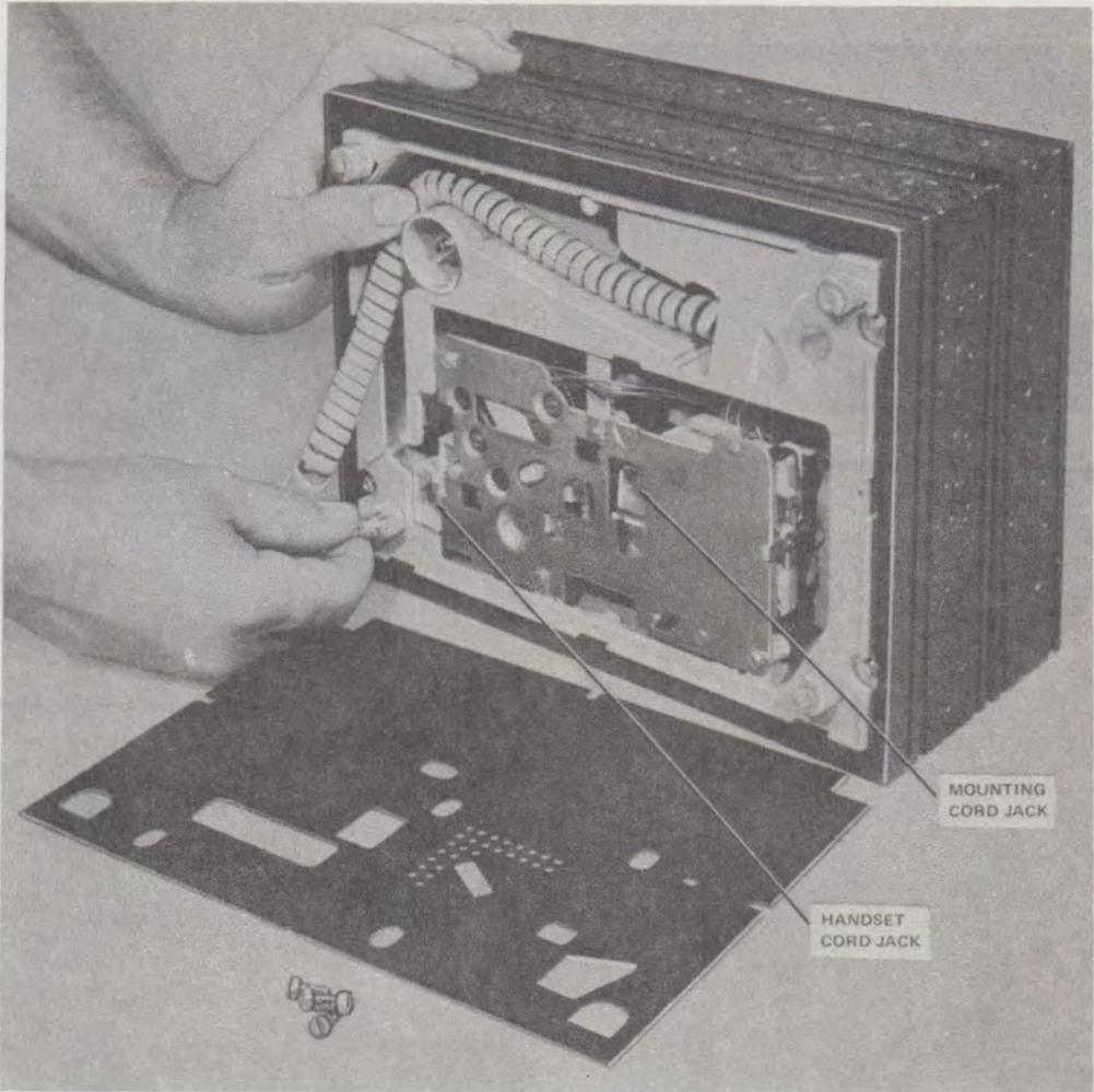
Fig. 7—Location of Handset and Mounting Cord Jacks
